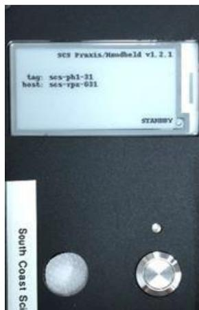
In standby mode, the LED goes off, the wlan0: connection is lost & STANDBY is displayed. Press the power button to get it running again. After about 2 minutes, it should return to normal operation.
