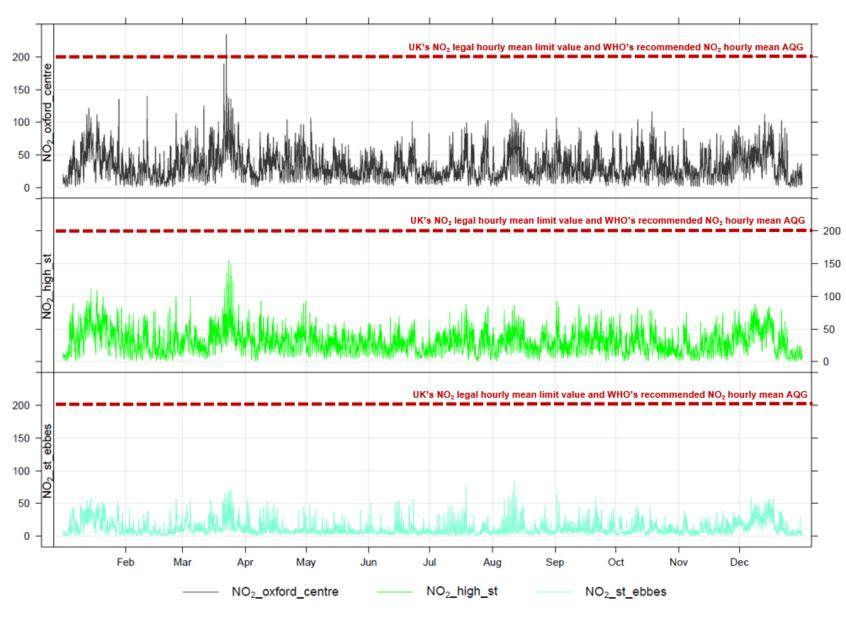
Figure 4 - Time series of hourly averaged concentrations of NO<sub>2</sub> (µg/m³) at automatic monitoring sites, 2022.
