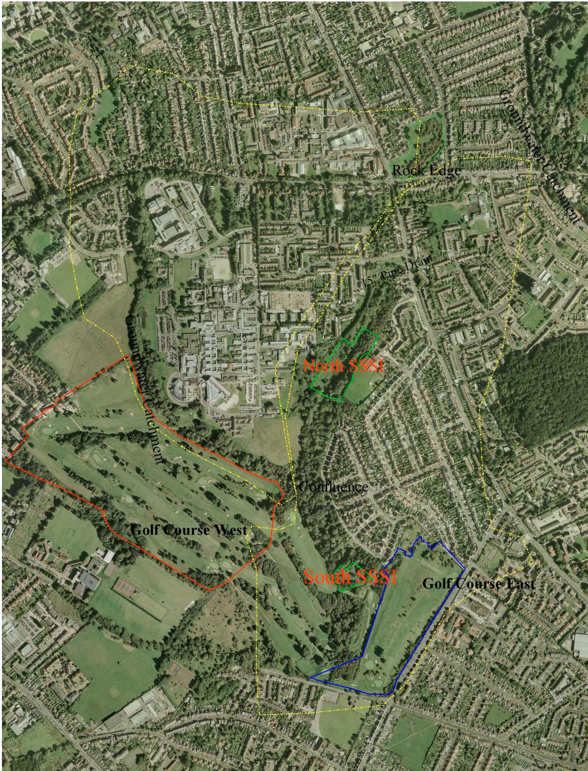
Figure 5 Groundwater catchment boundary marked in yellow for Boundary Brook to the confluence with the Lye Brook and the Lye Brook from source to the southern edge of the Golf Course.
