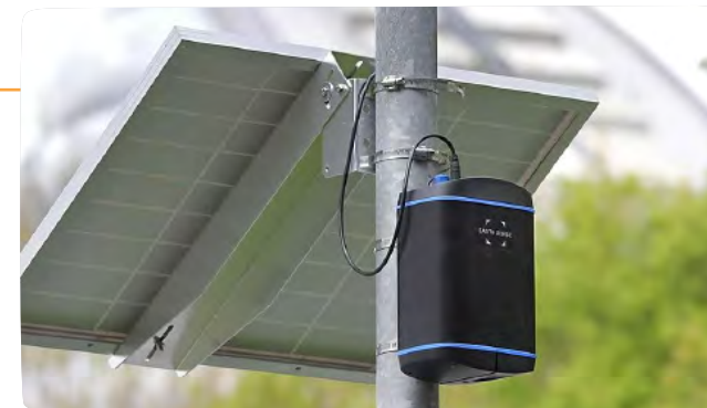
Street light with mounted air quality sensor.
