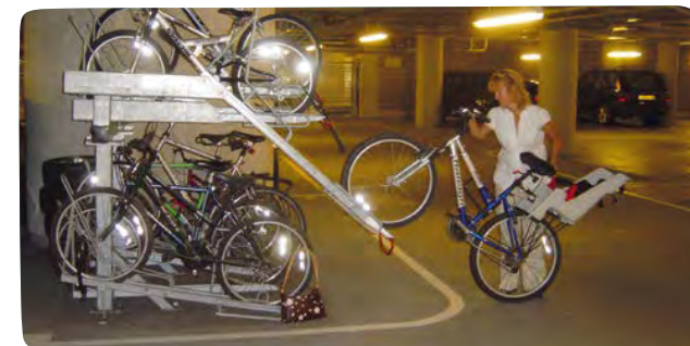
Secure communal apartment parking. Sheffield stands are preferred but alternatives may also be appropriate, subject to user, particularly where space is limited. The image at the bottom uses gas struts to aid lifting the upper tier
