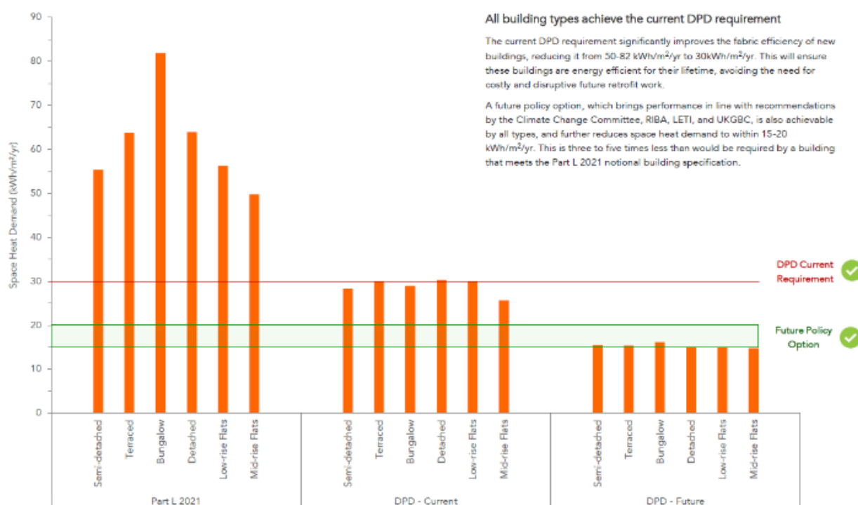
Figure 4.1: space heating performance of the six residential typologies assessed by Cornwall all able to meet stretching targets of 15-20 kWh/m 2 /yr (Cornwall Council, 2021).
