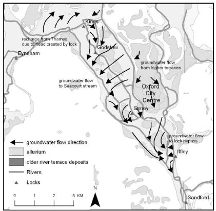
Figure 3.2 - Conceptual groundwater flow model for Oxford 15
