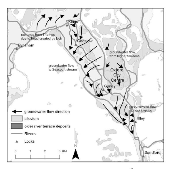
Figure 2.2: Conceptual groundwater flow model for Oxford (2007)<sup>44</sup>
