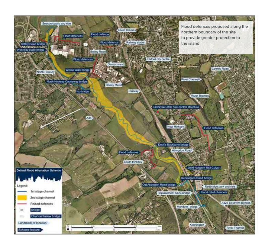
The height of the flood defences at this location (circled in red) is constrained by the surrounding topography. The (Above Ordnance Datum) design height of the proposed flood defences is 56.70m AOD , the 100 year flood event is 56.75m AOD.
