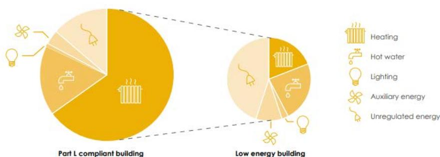
Figure 3: A low energy building attributes a smaller amount of its energy consumption for heating
