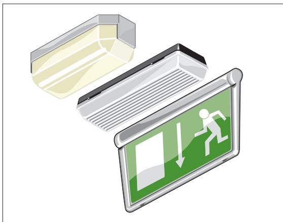
Single 'stand-alone' emergency escape lighting units (luminaires) may be sufficient in a marquee or other temporary structure and these can sometimes be combined with exit or directional signs (see Figure 22). The
